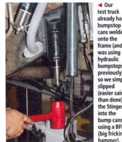
▲ The Stingers are completely (and easily) rebuildable and come apart in just a few minutes. Each Stinger comes with an internal spacer that you can put on the shaft to lower the travel to around 2.5 inches. Upon using the internal spacer, only two EVS foam cushions will be used on top of the shaft.
