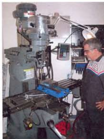
▶▶ Since we were installing these Stingers at OC Tranny while the truck was on a rack getting a new transmission, David Dibbs took the time to use his new mill to make us some plates. The plates were used to bolt the rear Stingers up into the factory bumpstop location on the frame.
