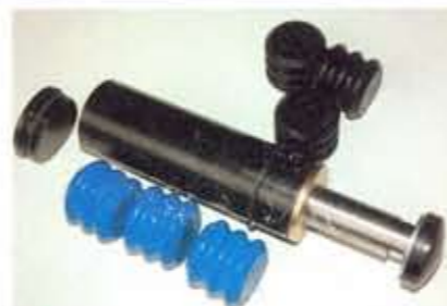
▲ The Daystar Stingers fit in a conventional 2-inch weld-on bumpstop can. They have four inches of travel and use three EVS foam cushions to slow down (and eventually stop) the compression of the bumpstop shaft. Each Stinger bumpstop comes with three blue EVS foam cushions and three black ones. The blue ones are softer and the black ones are harder. You can mix and match to get your desired bump effect.
