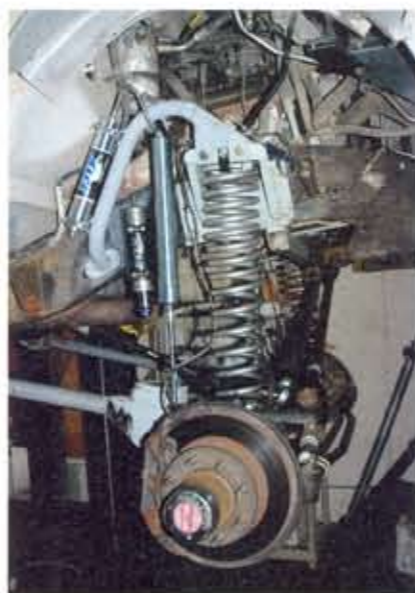
▲ Our test truck of choice was a 2002 Chevy 2500 4x4 with a CAGE Offroad solid axle swap kit and a Dana 60 axle. Off Road Evolution modified the shock hoops to accept the 2.0 Fox shocks and added bumpstop cans that previously held hydraulic bumpstops before we swapped them out for Daystar Stinger bumpstops.
