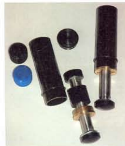
▲ The Stingers are completely (and easily) rebuildable and come apart in just a few minutes. Each Stinger comes with an internal spacer that you can put on the shaft to lower the travel to around 2.5 inches. Upon using the internal spacer, only two EVS foam cushions will be used on top of the shaft.
