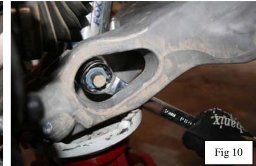
5. Loosen the upper ball joint nut but leave the nut in place by a couple of threads. Place pressure to the lower control arm using your jack. With the upper ball joint nut loose, strike the knuckle where the ball joint sits to loosen it from its mount. You will know when the ball joint is loose when it pops. Remove the ball joint nut and swing the upper control arm away from the knuckle.
