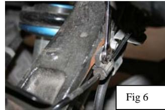
3. Loosen and remove the sway bar nut that is attaching the end link to the sway bar. Loosen and remove the outer tie rod; you will want to leave the nut on by a couple of threads, strike the side of the tie rod mount to free it, then remove the nut the rest of the way. Fig 7-8
